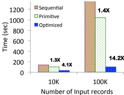
Figure 1: Total execution times of the sequential, naive and optimized implementations on ADAPT\_T1. Sequential code is run on a small EC2 instance; the map-reduced code is run on a large EC2 instance with 4 tasktracker nodes.
