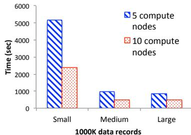
Figure 6: Performance on Small, Medium and Large instances for ADAPT\_T1 network with  $n=1,000K$ .
