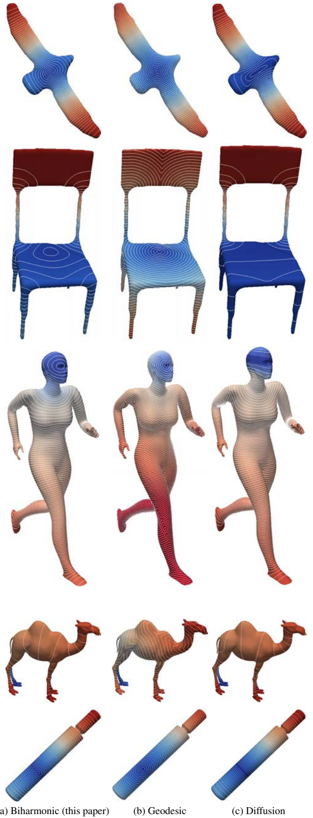
Fig. 5: Comparisons of biharmonic distance (left column) to geodesic (middle) and diffusion distances (right).
