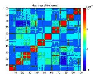
Heat map for the estimated kernel (the vertices are reordered to reveal the clusters of the graph)
