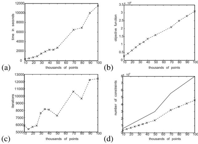
**Fig. 5.** The MFNU performance, a)Scaling of the MFNU b)Maximization results of the Maximum Furthest Neighbors objective c)Iterations required for the optimization d)Number of constrained  $kN$  (solid line), consolidated constraints (dashed line)
